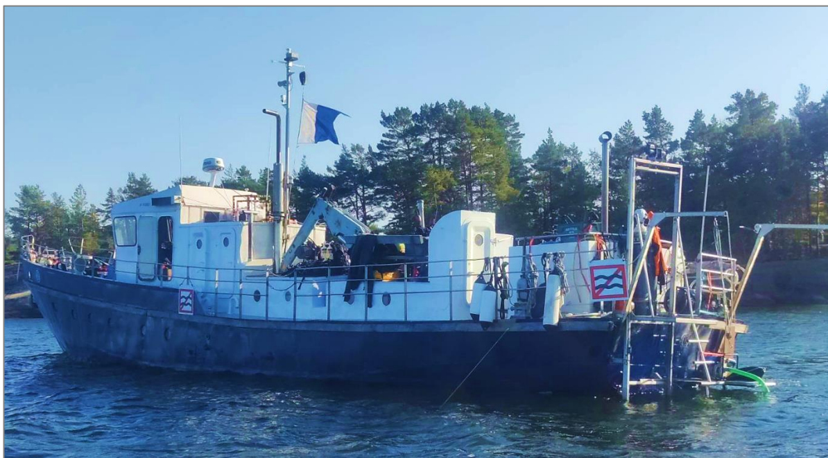
MAS's flagship DSV Stella anchored on the shore of Hamnholmarna. At the stern of the vessel, is a diver lift and next to it on the swimming platform an ejector pump and its suction hose. "No waves" signs are useful.
